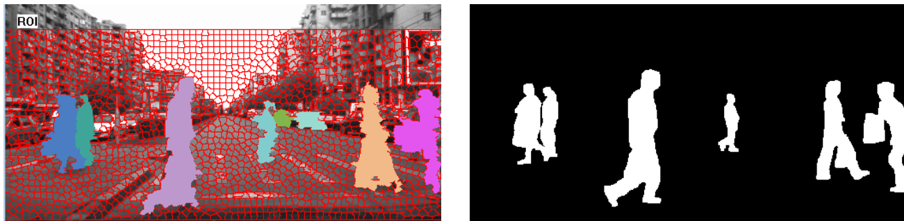
Figure 12. Evaluation method for one frame: left – obstacle detection result, right – manually labeled ground truth
